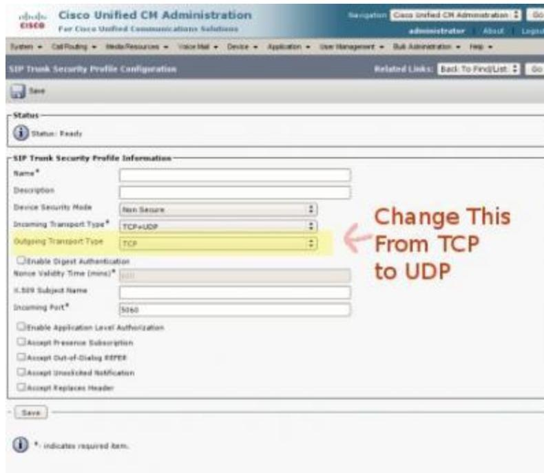
The screenshot shows the Cisco Unified CM Administration interface for configuring a SIP Trunk Security Profile. The 'Outgoing Transport Type' dropdown menu is highlighted in yellow and currently shows 'TCP'. A red arrow points to this dropdown with the text 'Change This From TCP to UDP'. Other fields include Name, Description, Device Security Mode (set to 'Non Secure'), Incoming Transport Type (set to 'TCP+UDP'), and various checkboxes for authentication and application level authorization.
