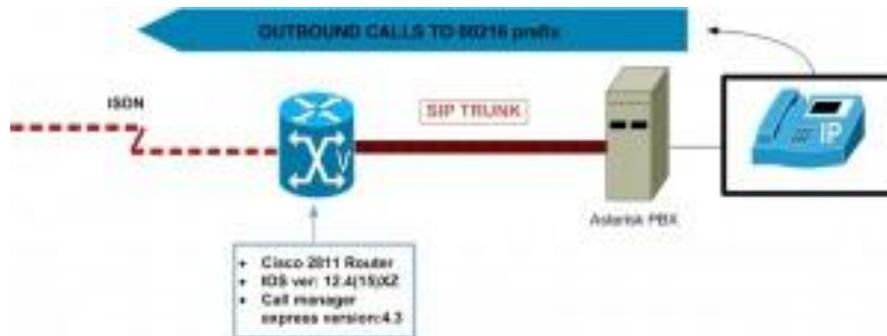
Here is instruction on how to integrate asterisk with Cisco Call Manager using SIP trunk.
